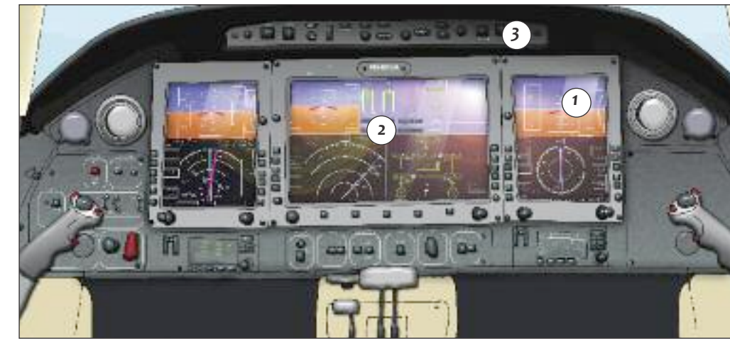
The controls in a light aircraft (below). The Primary Flight Display (1) shows altitude, speed and angle. A Multi-Function Display (2) monitors systems and engines. An Autopilot Control Panel (3) is used by the pilot to set course, speed and altitude.
