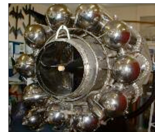
Power Jets W.2, a turbojet engine developed by Frank Whittle in the early 1940s.
